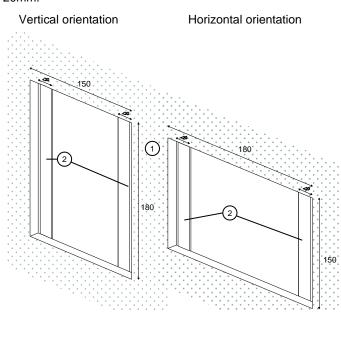
In the upper part of the device rear side, separate the frame of the device with a screwdriver near the groove (1) and push back the frame (3). Repeat the operation in the other upper groove (2). Remove the frame.
