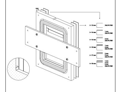
Place the accessory into the hole and adjust the exact horizontal (or vertical) position with the help of a level.
