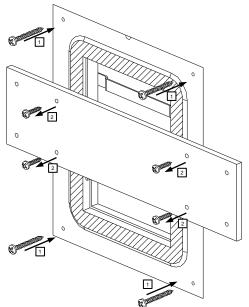
Plastering works must be done avoiding the *even surface*. Once the plaster is dry, wall painting and finishing works can be done (*accessory internal area* must not be painted)
