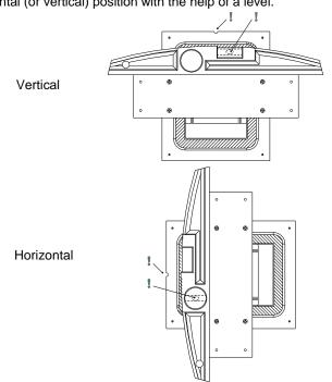
**5** Fix the accessory to the dry-wall frames with suitable screws (not included) [1]. Once fixed, the *auxiliary mounting part* can be removed by taking the four screws off [2].
