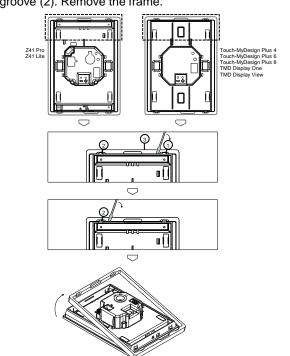
**3** Paste the necessary *rear supplements* to make the accessory and the drywall thickness match.
