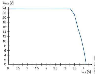
Output curve at  $T_a = 25\text{ }^\circ\text{C}$
