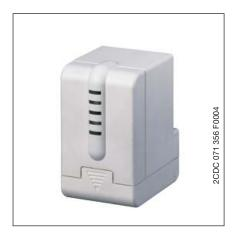
The Electromotor Valve Drive ST/K 1.1 is a proportional valve drive for controlling heating valves via the ABB i-bus<sup>®</sup> KNX. The valve drive is mounted on thermostat valve bases. The control is carried out via a continuous KNX room thermostat. The Electromotor Valve Drive ST/K 1.1 also has two binary inputs which can be used e.g. for the connection of a presence contact and/or window contact. The status of these inputs can be sent on the bus.
